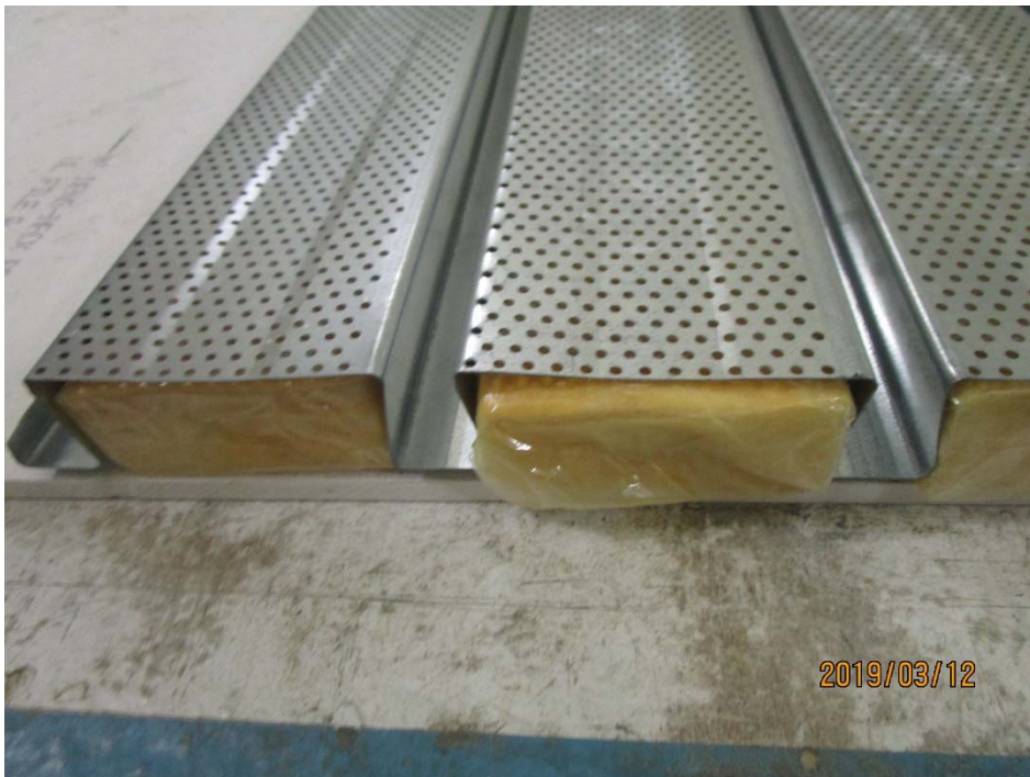
Figure 2 – Detail of specimen composition
