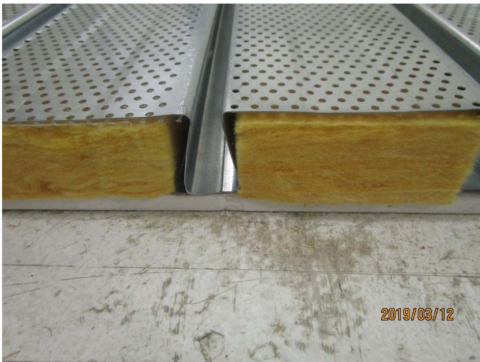
Figure 2 – Detail of specimen composition
