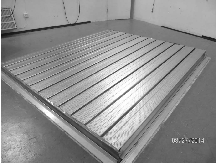
Figure 1 - Specimen mounted in the test chamber.
