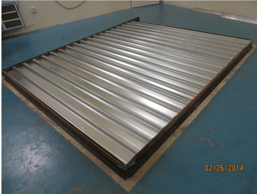
Figure 1 - Specimen mounted in the test chamber.
