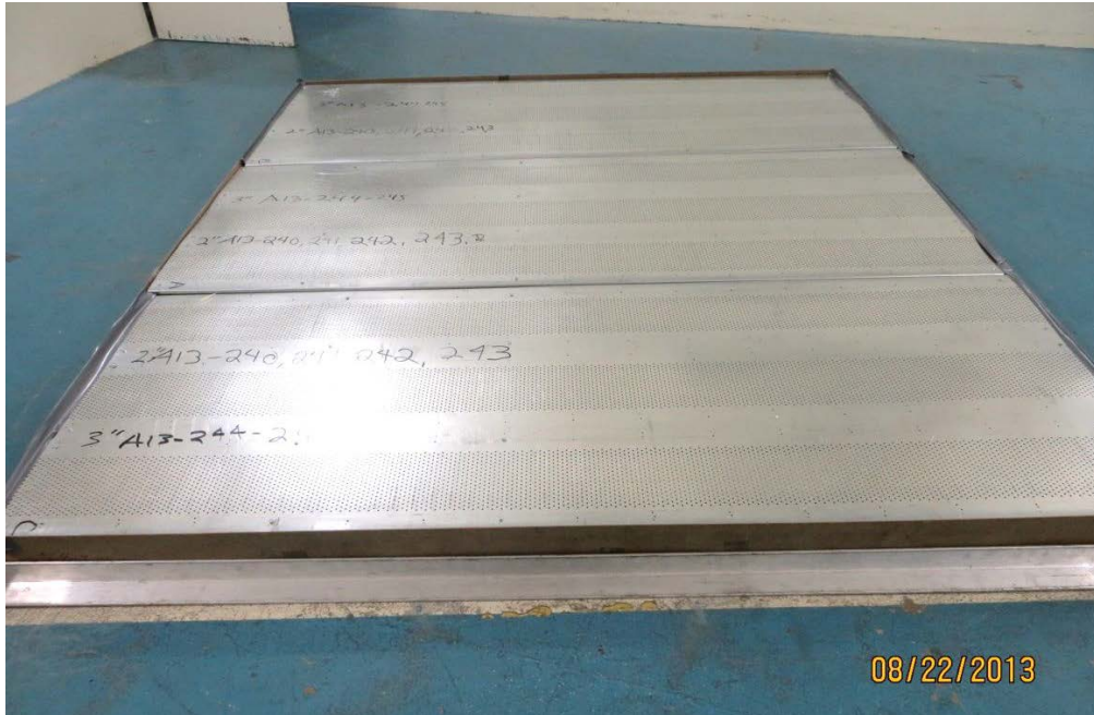
Figure 3 - Specimen mounted in the test chamber.
