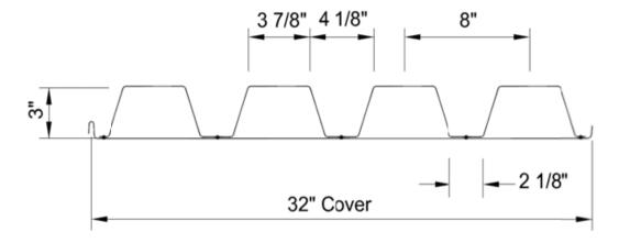
Figure 1 - Deck Section Detail (supplied by client).
