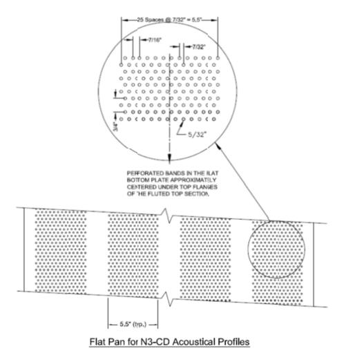
Figure 2 - Acoustical perforation detail (supplied by client).
