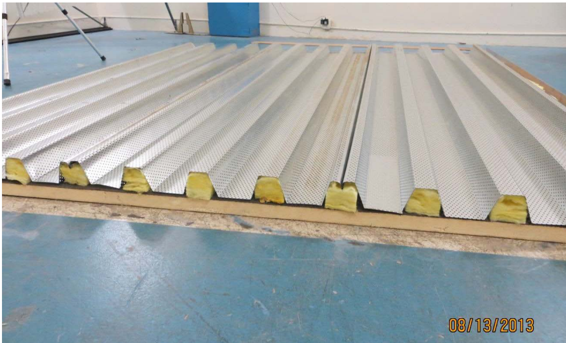
Figure 4 - Detail of the test specimen.
