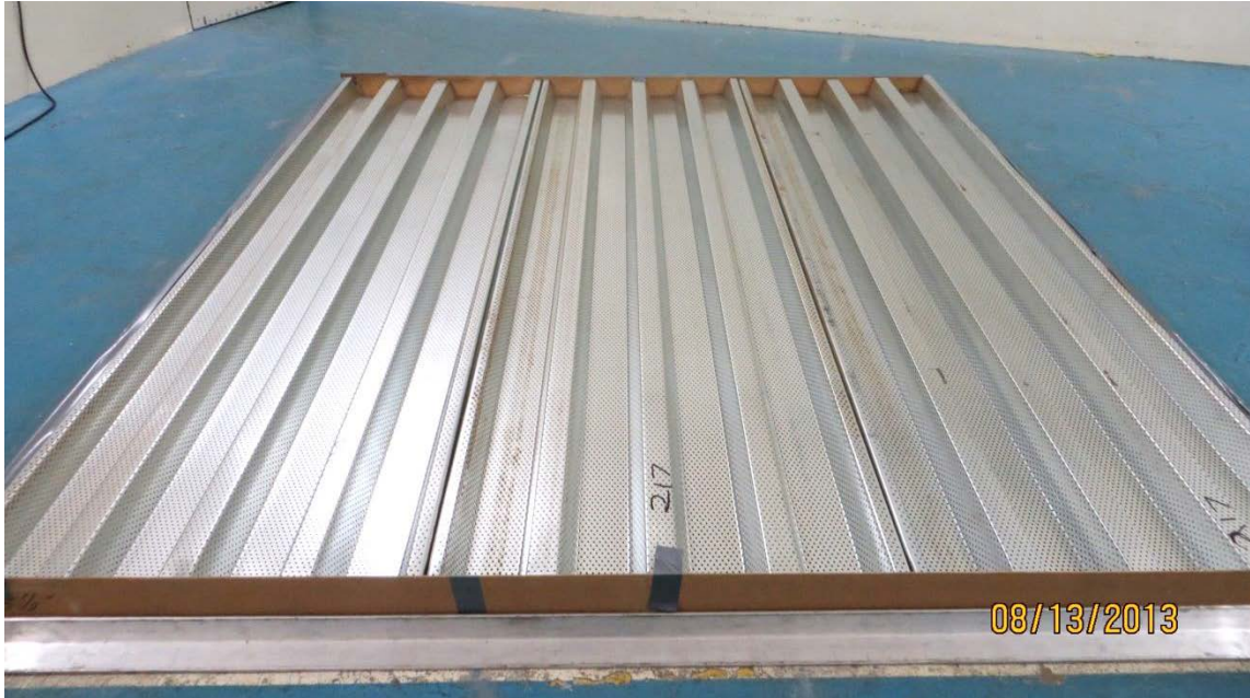
Figure 3 - Specimen mounted in the test chamber.
